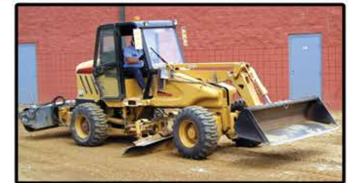
With 45 degrees of Moldboard Tilt, the M415 is perfect for blue-topping parking lots, driveways and shoulders.
